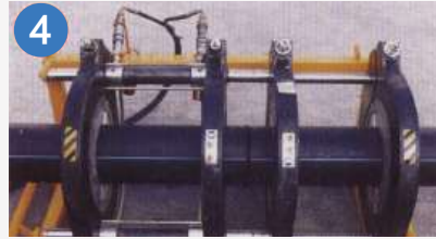
④ After the heating is completed, the heating plate is taken out, and the two heating surfaces are quickly joined, and the pressure is raised to the welding pressure and kept cool.
